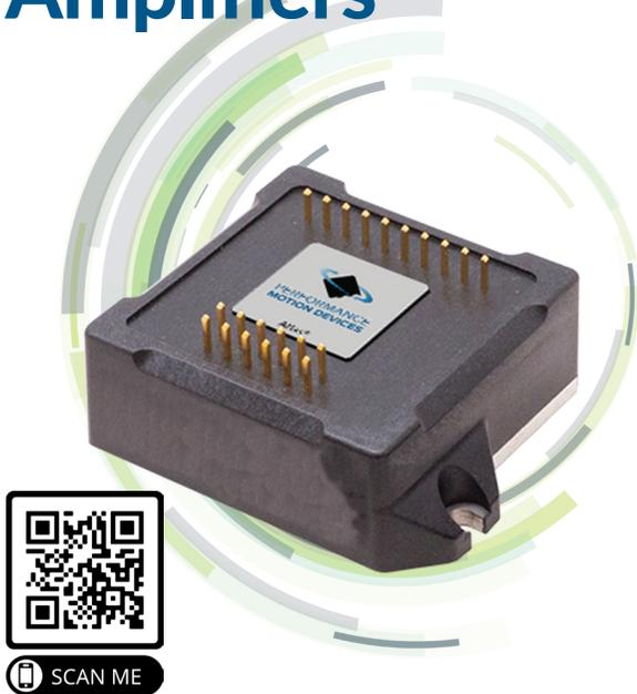
**ATLAS® Digital Amplifiers** are compact single-axis amplifiers that provide high performance torque control for DC Brush, Brushless DC, and step motors. They are packaged in a compact, solderable module and are ideal for use in positioning motion control, velocity control, and precision force control applications.
