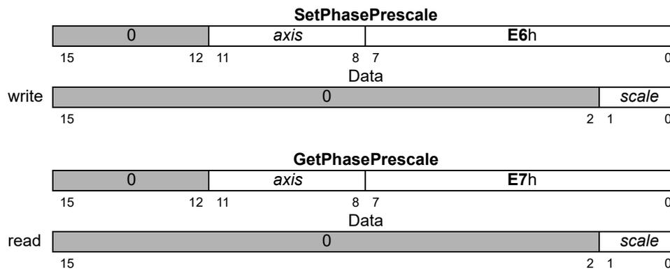
**Description**            **SetPhasePrescale** controls scaling of the encoder counts before they are used to calculate a commutation angle for the specified *axis*. When operated in the pre-scale mode, the motion control IC can commutate motors with a high number of counts per electrical cycle, such as motors with very high accuracy encoders.
