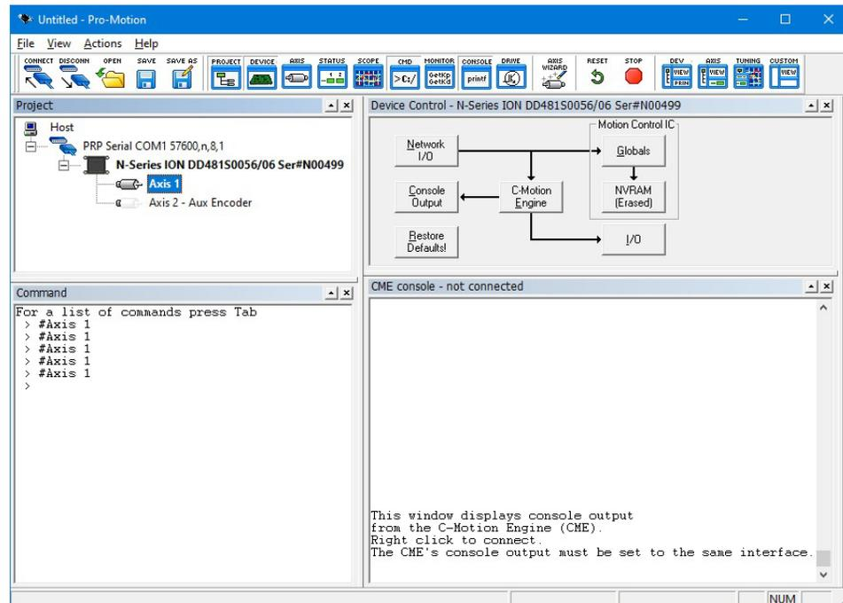
At the center of the screen you will see the **Device Control** window. This convenient graphical representation of the CME device allows you to manage card-level functions. The **Console** window is to the bottom. This will show messages output from the C-Motion Engine.
